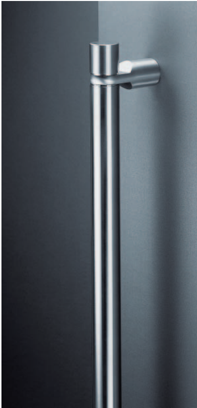
Sembla 1729 38øx692x100mm Sembla pull handle with Drum tips both ends. Bolt through fixings. Fixing centres at 600mm. Finishes: SS • PS • MA
