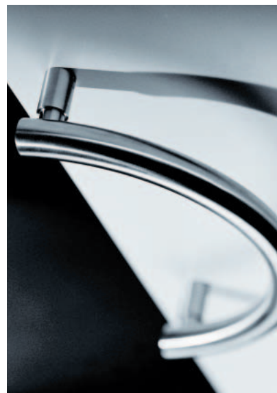
Mode 1335 38øx463x223mm Semicircular pull handle, single, with bolt through fixings. 90mm projection. Fixing centres at 425mm. Finishes: SS • PS • TA • PB • PZ
