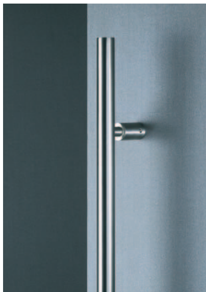
1751 20øx750x67mm Pull handle with bolt through fixings. Fixing centres at 600mm. Finishes: SS • PS
